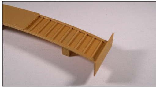
Figure 14. 3D printed spoiler for Design Concept 5 using PLA/metal composite filament
