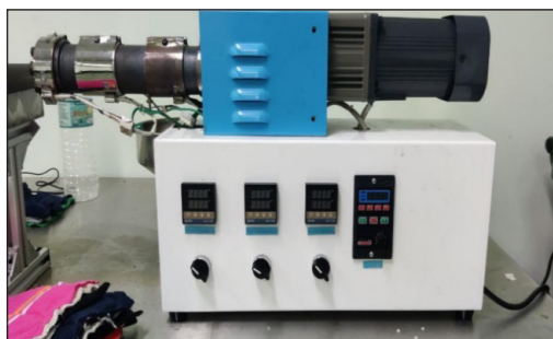
Figure 2. Single screw extruder machine used in this study
